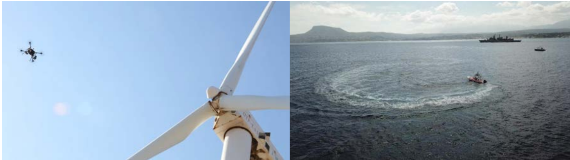
Figure 13: Perceptual Robotics Unmanned Air Vehicle inspecting a wind turbine (left). Altus LSA Unmanned Surface Vehicle for maritime perimeter patrol (right)
