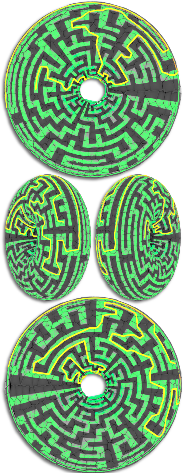
Figure 7. The “torus” environment. The torus constraint manifold (grey) with an overlaid obstacle maze and atlas. The resulting graph (green) of a run of atlas-based PRM along with a solution path (yellow) is shown on the torus.
